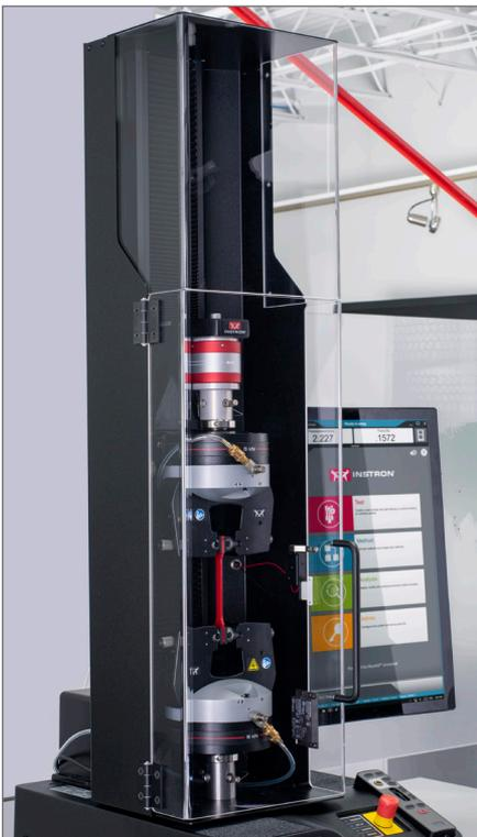
Single Column Shield Fully Encloses Test Space
