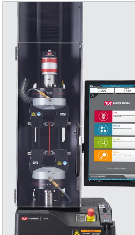
Single Column Shield Fully Encloses Test Space
