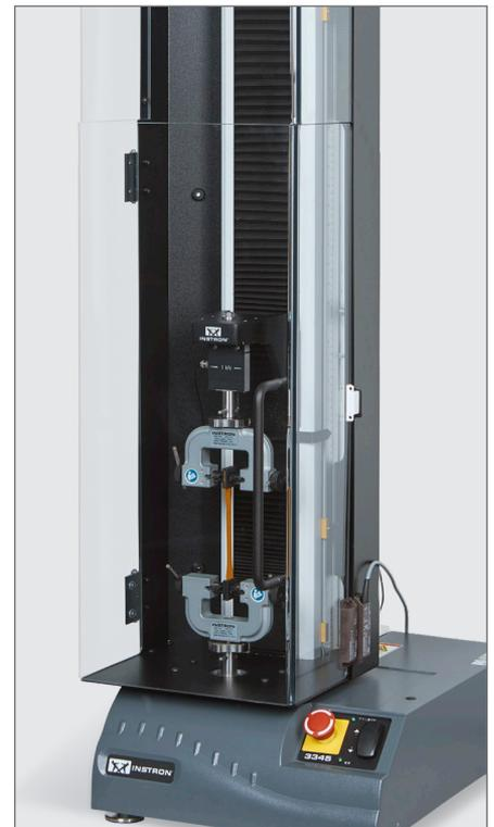
Single Column Shield Fully Encloses Test Space
