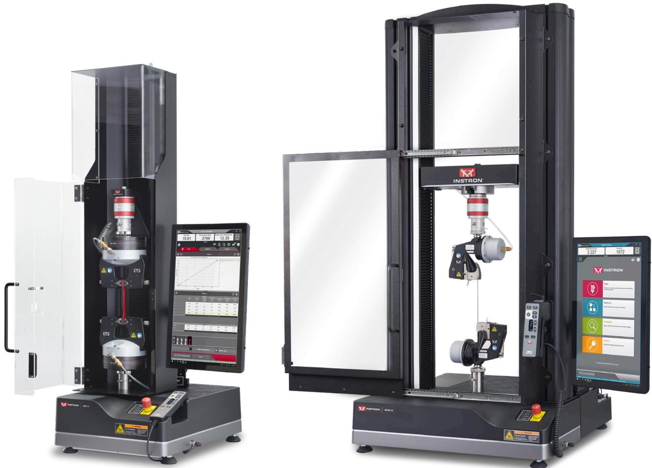
Instron® materials testing systems are designed to be as safe as possible, but some applications can pose dangers to operators because of debris or potential pinch hazards. To protect operators without decreasing usability, Instron has developed new shields for tabletop and single column systems. These shields have been designed to optimize safety, ease of use, and laboratory space.
