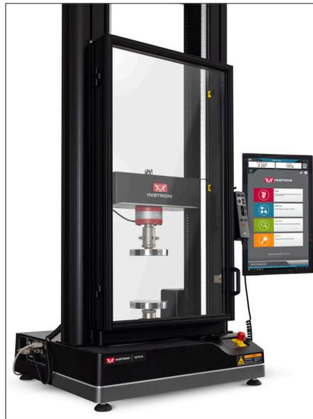
Debris Shield on a Table Mounted System
