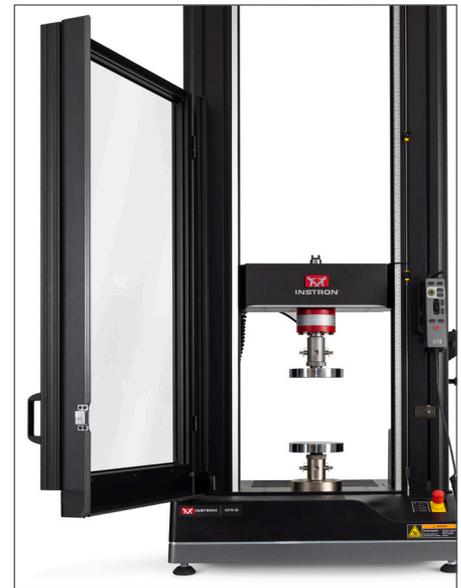
Debris Shield open on a Table Mounted System
