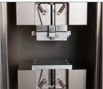
"Piggy Back" Adaptors Allow Fixtures to be Installed without the Need to Remove the Grips from the Machine
