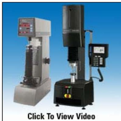
been developed as an alternative method of load application. Closed-loop testers use a force measuring device (a load cell), instead of a stack of weights, to measure and regulate the applied force by a motorized actuator. This system constantly monitors and adjusts the applied force, virtually eliminating force errors and increasing tester accuracy and repeatability.
