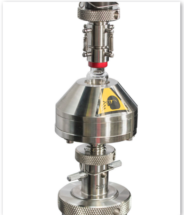
Figure 2: Vial specimen being tested on a 5965 with a 100 N load cell.
