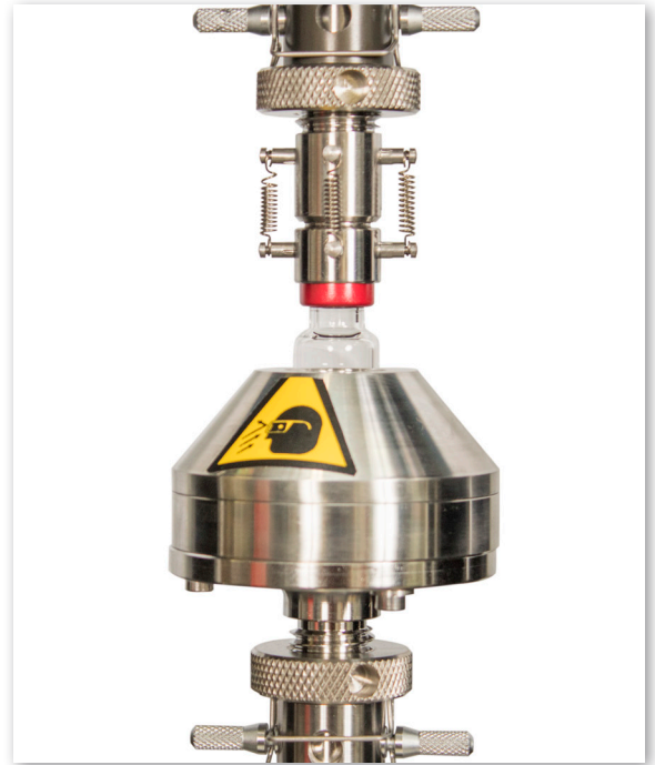
Figure 1: Vial specimen positioned between platens before start of test.
